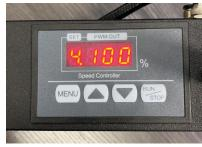
Press menu button to get to **SET 4**, then use the arrows to set the number to 100. This is the fastest speed.
