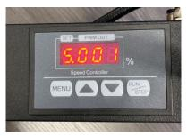
Press menu button to get to **SET 5**, then use the arrows to set the number to 1. This sets the steps of speed change when using the up/down arrows. (Options to jump are 1, 2, 5, 10)
